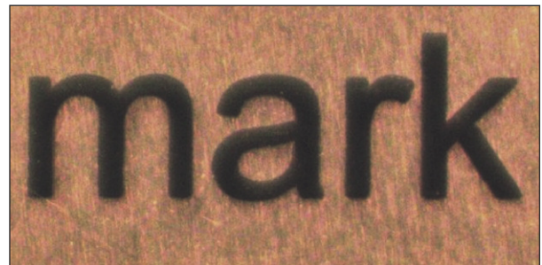
Mark on 17-4 autoclaved and passivated stainless steel
