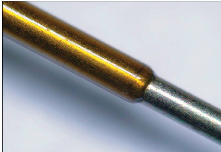
Figure 2 CO 2 laser stripping of polyimide wire insulation
