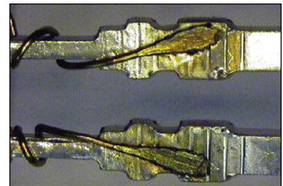
Magnet wire to terminal
