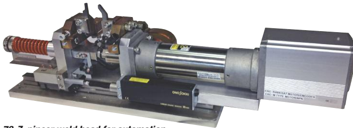
73-Z, pincer weld head for automation
