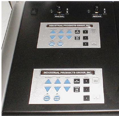
**FIGURE 3.** Microweld station includes three IPG camera controllers in addition to the three TruView cameras. The controllers can store up to three individual focus, brightness, and zoom settings for different weld locations for systems that are not PC based, while the ProCheck software can store an additional 99 settings, if necessary.
