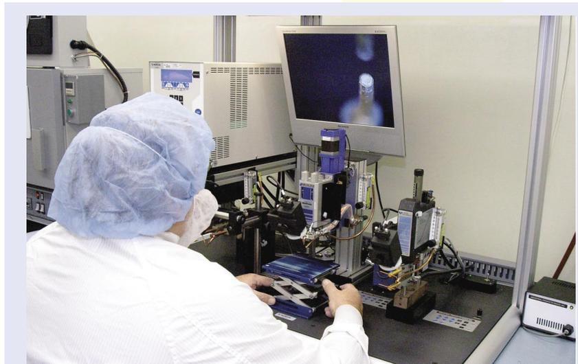
**FIGURE 1.** Multihead microweld station developed by Miyachi Unitek and Industrial Products Group for Medtronic uses ProCheck software and closed-loop, weld-head feedback control to perform multiple microwelds on a pacemaker.
