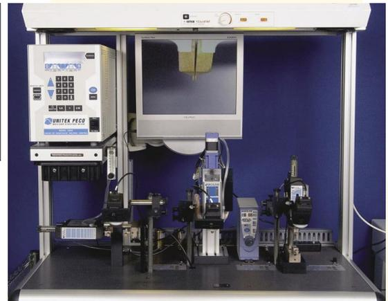
tall, which is useful for machine-vision workstation retrofit. The stage comes with a clear Lexan window for backlighting; however, the microweld station requires direct illumination so the technician can see the weld location and the approaching weld head.
