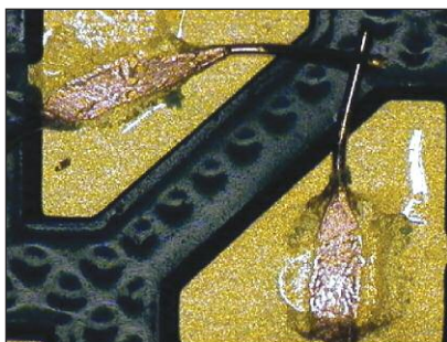
0.005 in diameter magnet wire to gold pad
