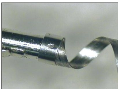
0.002 in thick platinum strip to platinum tube
