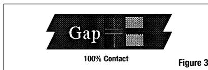
Figure 3 shows a Unitip electrode tip face correctly centered on a printed circuit trace with electrode gap parallel to the trace.
