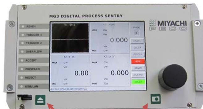
Press both touch buttons simultaneously max 10 sec. for a shutdown.
