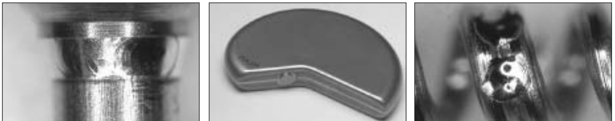
Common applications include welding end effector tools to tube bodies, hermetically sealing implantable devices, and spot welding on catheter coils used for balloon or stent placement.
