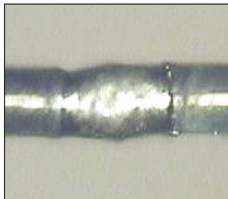
Guide wire welding
