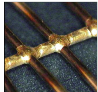
Small gauge wire welding
