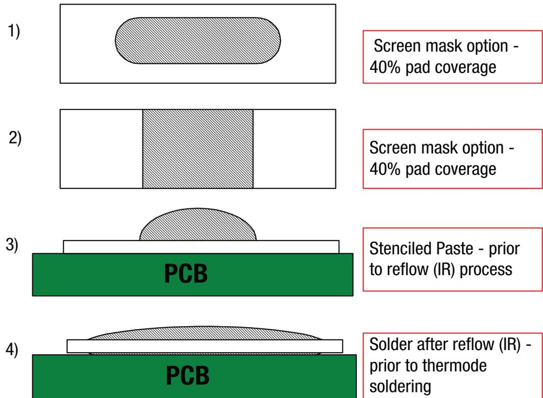
1) A smaller screen aperture can provide 40% solder coverage of pad.
