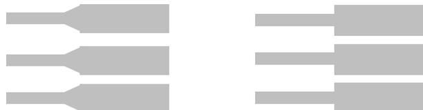
For multi-layer boards, restrict the traces under the bonding area to the smallest width (signal) traces and spread equally under the pads on the PCB. Any shielding on the PCB should have an equal effect along the joint area.
