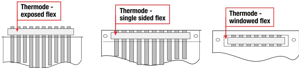
**Thermode Width:** For the best thermal performance and lifetime of the thermode, the minimum size should be 0.059". The standard size is 0.079", due to better performance and longevity. Where solder amounts are not well controlled or room is limited, it is possible to use a 0.047" wide thermode however thermode life and performance will be reduced.
