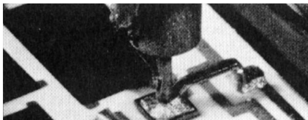
A 17P20 peg tip thermode reflow solders a plated contact and bus bar to pads on ceramic substrate.
