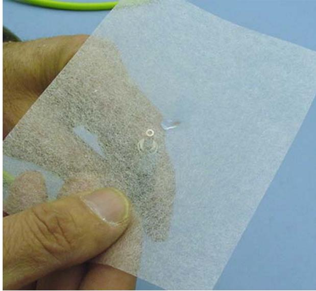
8. If the fiber end is still dirty, then fold a new piece of lens cleaning paper three times to make a rigid “cleaning” corner. Place a drop of acetone on the “cleaning” corner, and gently rub the fiber end. Concentrate the rubbing action to the middle of the fiber (core) and avoid rubbing the connector body. Repeat steps 5 and 6 and re-inspect the fiber end with the fiber end scope. If it is clean continue with the other end of the cable, else repeat this step until the fiber end is clean.
