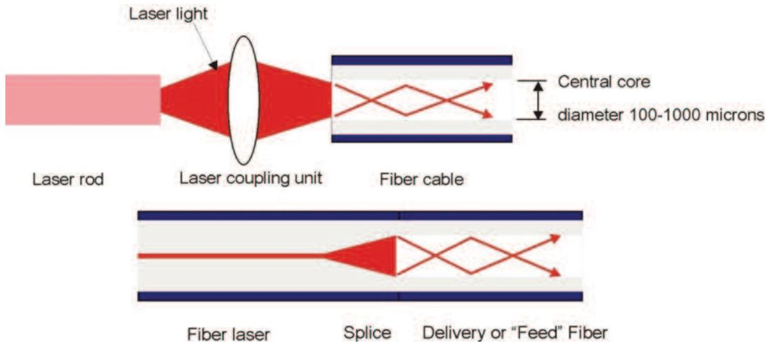
*Figure 2 – Options for launching laser into the fiber*
