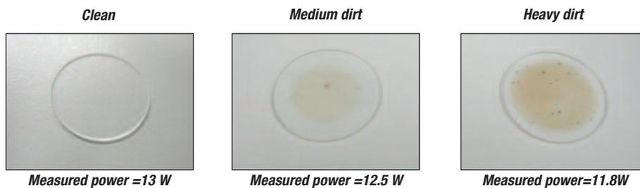
*Figure 6 – Effect of contamination on transmitted laser power*
