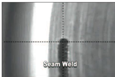
*Figure 4 – Through the lens viewing of part and process*
