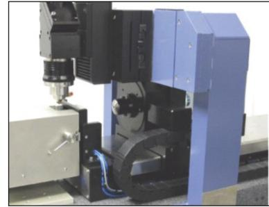
*Figure 7 – X and rotary plus YZ motion tube cutter*
