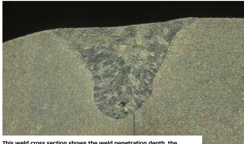
This weld cross section shows the weld penetration depth, the quality of the weld, and how the materials have melted together.
