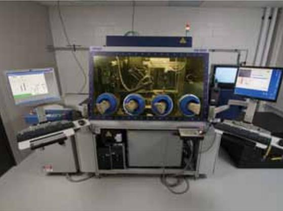
Shown here is an environmentally controlled glovebox for laser welding.
