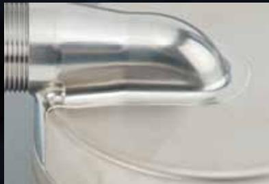
The device's 22 distinct seam welds include tiny, curved contours, shown here in a magnified view. These curves require quick, precise changes in laser beam positioning.
