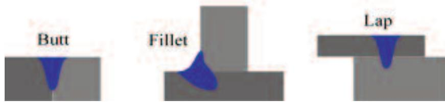
Figure 2 – Joint types for laser welding
