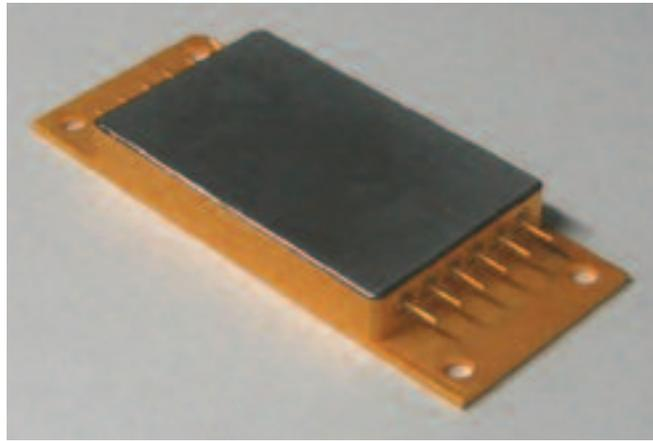
*Figure 1 – Laser seam sealed electronic package*
