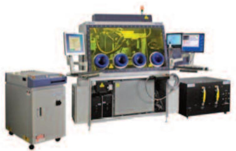
*Figure 3 – Example of a laser seam sealing system*
