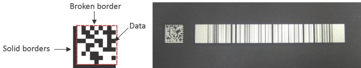
*The data is encoded in the light and dark “cells” contained within the red dotted square. A general size comparison between Data Matrix Code both containing “Unique Identification Marking” and barcode 39 shows the much higher data density of the DM code*
