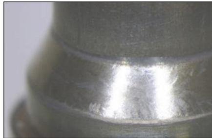
*Figure 4 – Conduction welding*
