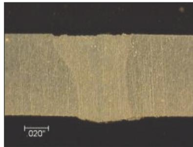
Aluminum bead on plate 0.06" thick at 60 IPM
