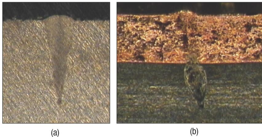
*Cross section of (a) 100 micron wide spot weld in steel (b) High power density is able to overcome reflectivity in seam welding 0.015-inch thick copper to steel at 600 IPM. To prevent issues with back reflection, the head is angled, which produces the angled weld.*
