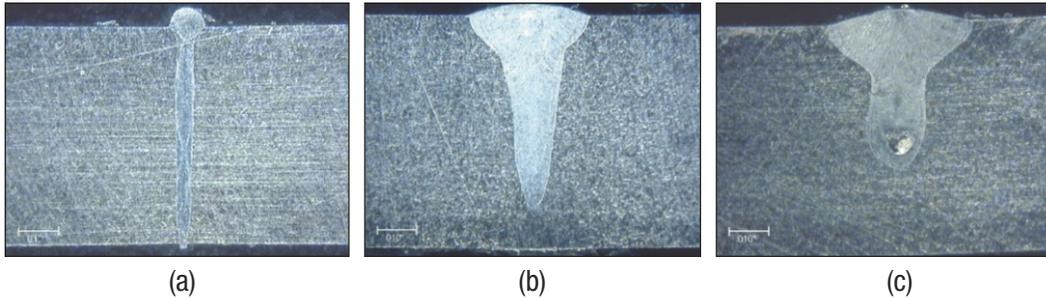
*Cross section in 0.06" thick stainless steel of (a) Single mode fiber laser at 500 W, 300 ipm with a 30 micron spot size (b) Multi mode laser at 700 W, 100 ipm with a 150 micron spot size (c) Multi mode fiber laser at 1 kW, 80 ipm with a 250 micron spot size.*
