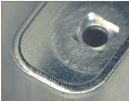
*Figure 1 – Seam welding of aluminum cans*
