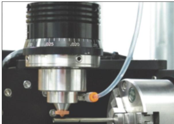
*Figure 3 – Interior of 5 axes multi-axis laser fusion cutting system*
