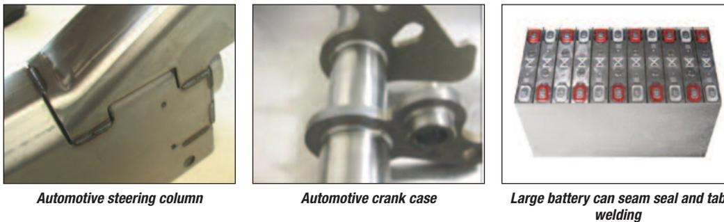
**Figure 2 – Examples of high power CW laser welding**
