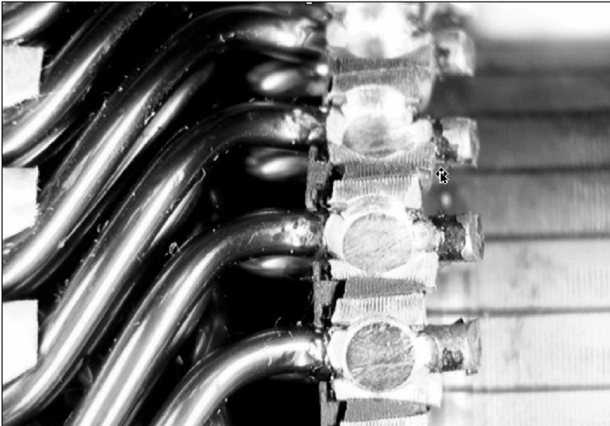
*Minimized burn back using AC Inverter*
