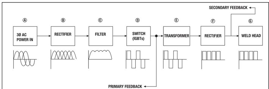
BLOCK C is the filtering stage. In this stage capacitors are used to filter out the noise and minimize the ripple effect left over from the rectification process. This cleans up the waveform and results in more consistent current. The capacitors do not act as a storage medium, as in Capacitive Discharge style machines, even though they do store energy during this rectification. It is advised to use safety precautions indicated by the manufacturer, due to the amount of energy that can be stored.
