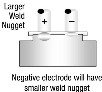
**Figure 3: Series welding of a battery tab to cell**
