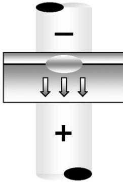
**Figure 2: Welding resistive parts of unequal thickness**
