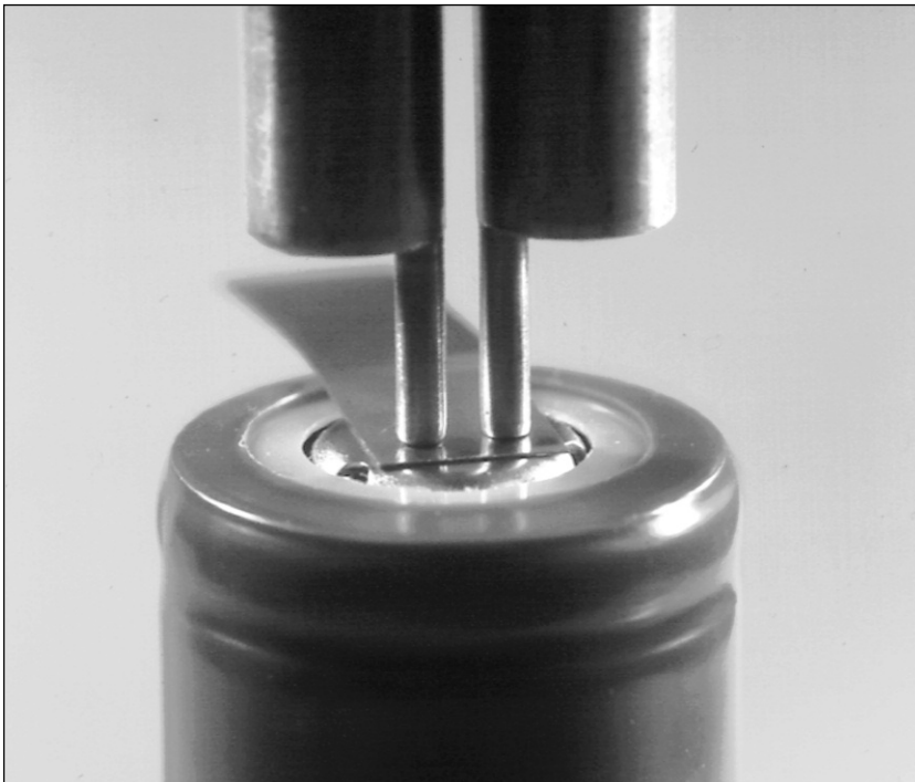
Figure 1: Nickel battery tab to nickel plated cold rolled steel battery cap using Constant Current mode. HF2 Power Supply, X11/4000A Transformer, 88A/24 Weld Head.
