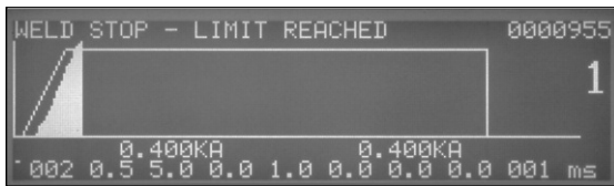
Figure 4: Energy limit function terminates weld when limit is reached
